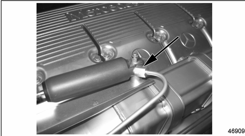
Figure 4 Air Supply Line to Throttle Shutoff Valve Actuator
