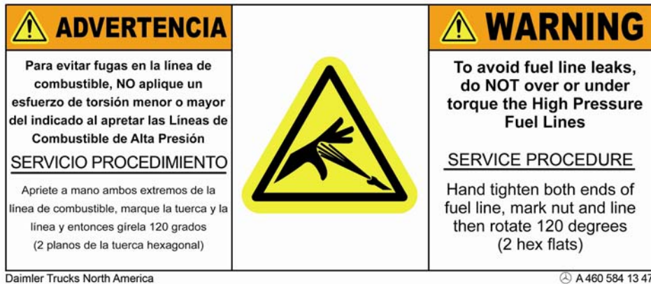
Figure 9 Installation of New Torque Specification Label on Intake Manifold
