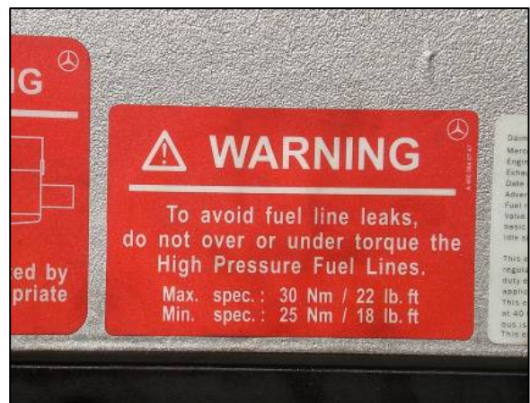
Figure 8 Removal of Red Torque Specification Label on Intake Manifold
