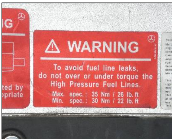
Figure 8 Removal of Red Torque Specification Label on Intake Manifold
