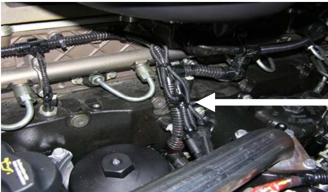
Figure 10 Installation of Adaptor Harness Using Tie Straps
