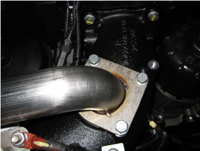
Figure 5 Installation of Mixer Pipe
