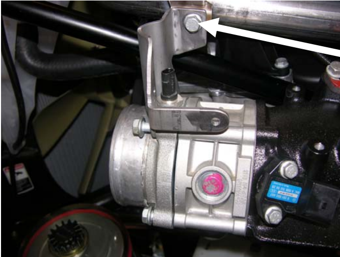
Figure 9 Installation of Intake Throttle Valve and Related Parts
