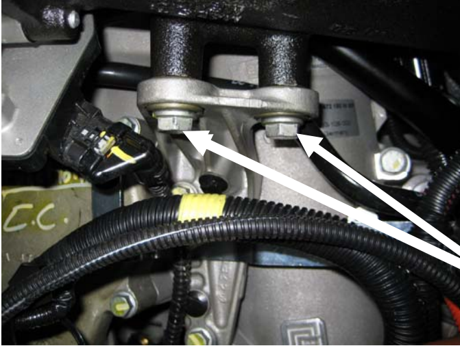
Figure 3 Cold Boost Pipe Bracket Bolts to Cold Boost Pipe
